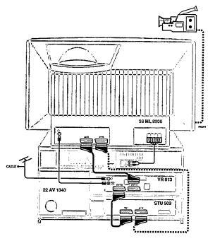
In order to make automatic recording and display of D2-MAC Wide-Screen (16:9) pictures possible, a special configuration is recommended as shown in the drawing.
